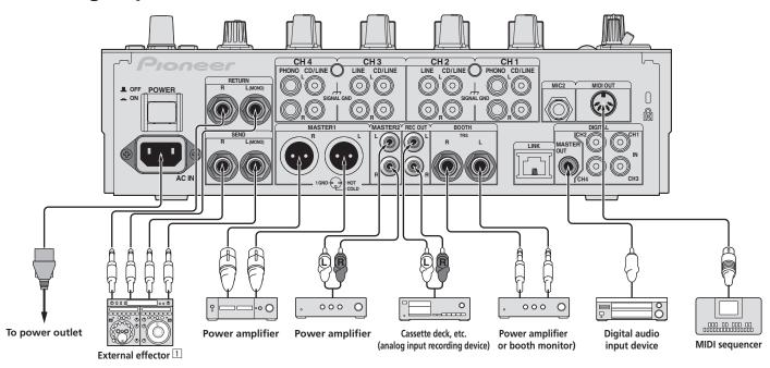
1 Also connect the external effector to the [RETURN] terminal (input terminal).
