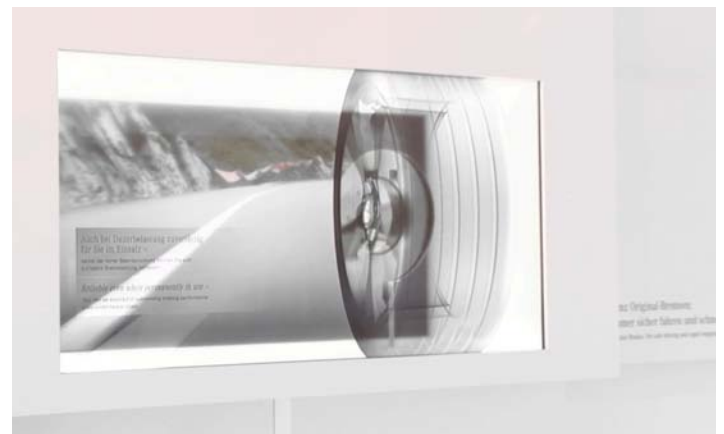
Application Possibility: 46" transparent LCD on a show stand with a conventional LCD in the background and an exhibit inbetween
