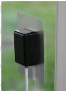
Stuck onto a chosen surface, the SensoPad detects approach of finger and triggers the associated action, plays a specific file or directory.
