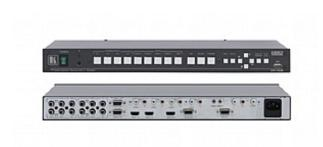
The VP-728 is a 9-input scaler/switcher for analog and digital video, unbalanced stereo, and S/PDIF audio signals. It up- or down-scales any video signal: composite, s-Video (Y/C), component video (YUV), HDMI, computer graphics video and JPEG files to a selectable graphics or HDTV output resolution via HDMI or 15-pin HD outputs. It provides glitch-free switching between sources through FTB™ (fade-thru-black) switching technology.
