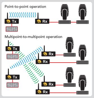
W-DMX is unique in its use of certain advanced radio techniques which are more often found in mobile phone and military communications. Rather than using fixed frequency channels, W-DMX uses adaptive frequency hopping technology (as well as TDMA and GFSK technques) to continually check for interference and to rapidly move operation over to clear radio channels. The frequency hops occur one thousand times every second to ensure smooth, efficient and robust operation.
