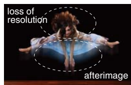
3D Noise Reduction Alone Afterimage and some loss of resolution is seen
