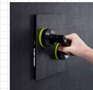
▲ The GEKKO is a specially designed tool enabling you to replace the LED modules at the front with ease. The control unit at the back also dismantles quickly thanks to two manual locks.
